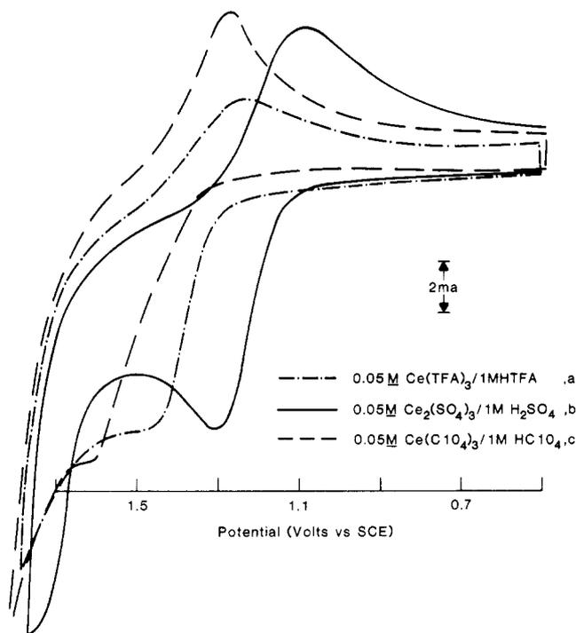
**Figure 1.** Cyclic voltammetric response of Ce(IV) at Pt in (a) 1 M HTFA, (b) 1 M H<sub>2</sub>SO<sub>4</sub>, (c) 1 M HClO<sub>4</sub>.
