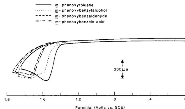
**Figure 2.** Cyclic voltammetric response of *m*-phenoxytoluene and derivatives in trifluoroacetic acid/acetonitrile/water (1/1/2) at glassy carbon.
