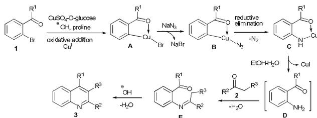
Scheme 1 Plausible mechanism for the synthesis of quinolines **3**.
