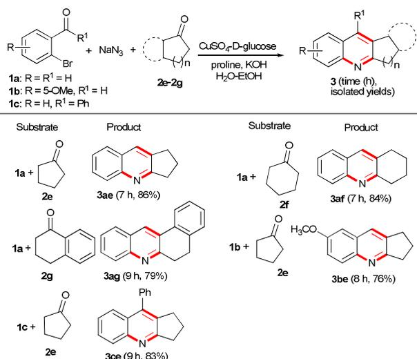
Under the optimal reaction conditions, the protocol scope and generality for the direct construction of quinolines **3** was explored (Table 2). The one-pot cascade process serves as a general approach to access valuable substituted/annulated quinolines in excellent yields (86-95%) with a broad substrate scope. 2-Bromobenzaldehydes (**1a-b**) and 2-bromobenzophenone (**1c**) reacted smoothly with both acyclic (**2a-b**) and cyclic (**2c-d**) 1,3-
