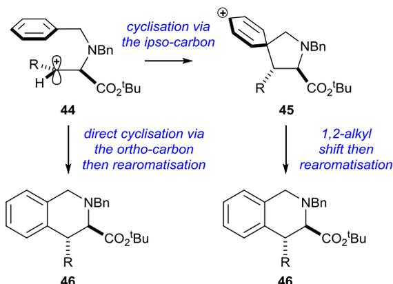
Fig. 5. Possible mechanisms for cyclisation to give tetrahydroisoquinolines. [R=aryl].
