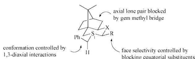
in the new *in situ* process. In the design of new catalysts we were guided by our experiences using oxathiane **1**, from which we learnt that three features were required to achieve good enantiocontrol. These comprised: (i) formation of a single sulfur ylide by blocking one of the two sulfur lone pairs, (ii) control in the conformation of the ylide and (iii) control in the face selectivity of the ylide (Fig. 1).
