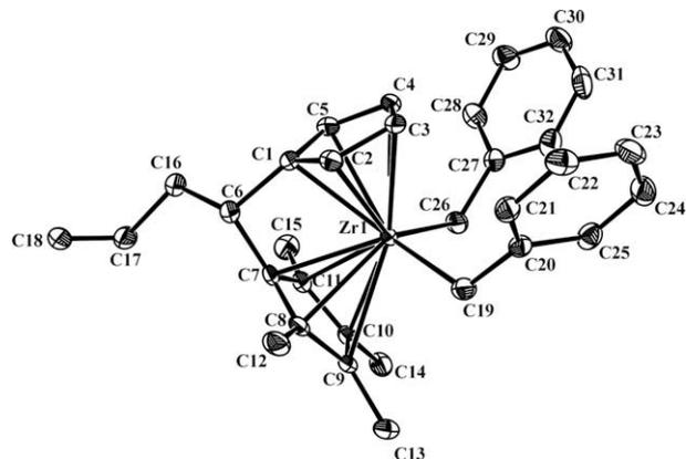
**Fig. 2.** Molecular structure and atom labelling scheme for  $[\text{Zr}\{(\text{CH}_2=\text{CHCH}_2)\text{CH}(\eta^5\text{-C}_5\text{Me}_4)(\eta^5\text{-C}_5\text{H}_4)\}(\text{CH}_2\text{Ph})_2]$  (**11**) with thermal ellipsoids at the 30% probability.
