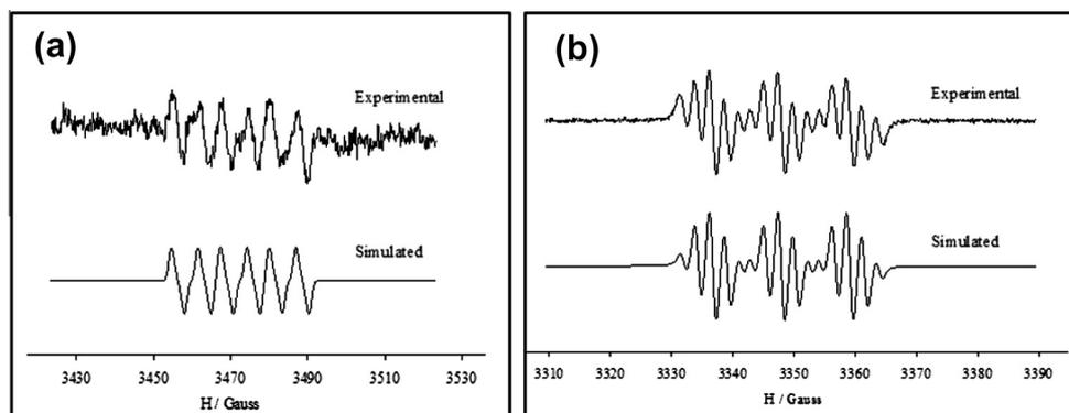
**Figure 1.** Experimental and simulated EPR spectra of (a) the TMPO adduct resulting from the reaction of TFE with PhNCO in the presence of TMPO, and (b) MNP and B (Scheme 2) adduct.
