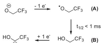
**Scheme 2.** Proposed voltammetric cycle for  $\text{CF}_3\text{CH}_2\text{ONa}$ .
