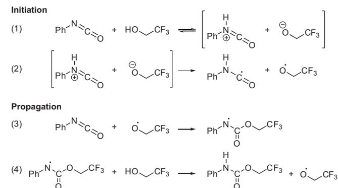
**Scheme 3.** Proposed radical chain mechanism for the reaction of TFE with phenylisocyanate.
