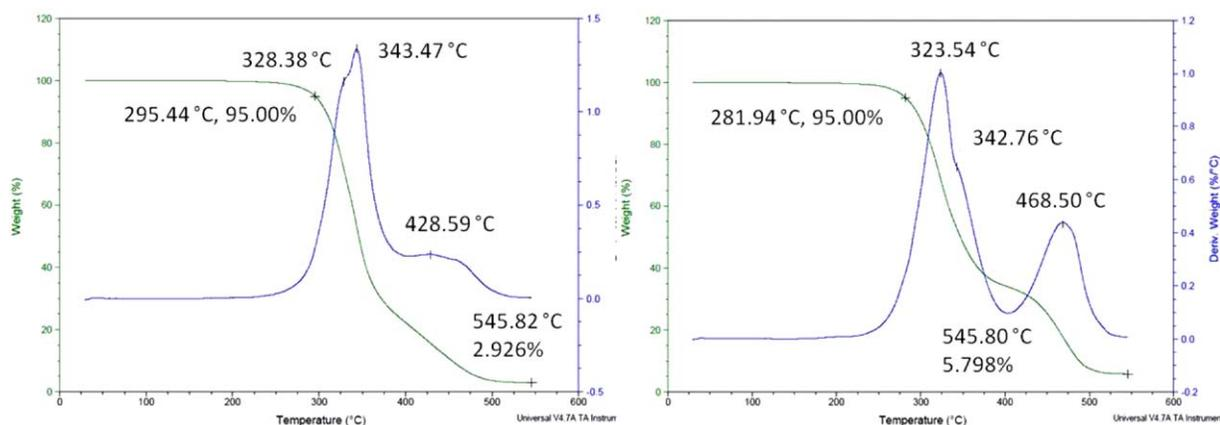
**FIGURE 7** TGA chromatograms of PU1 (left) and PU2 (right) under nitrogen. [Color figure can be viewed in the online issue, which is available at [wileyonlinelibrary.com](http://wileyonlinelibrary.com).]
