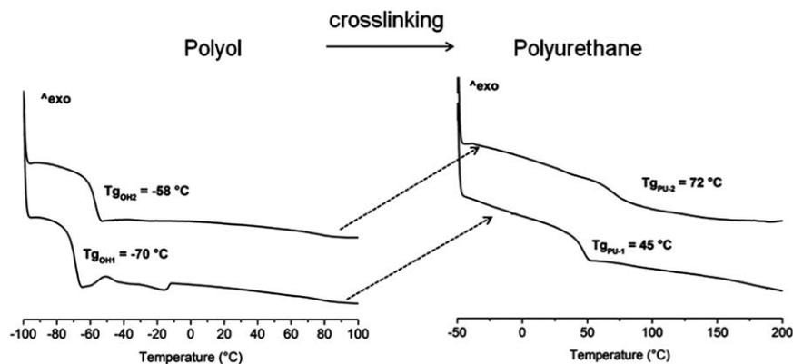
**FIGURE 6** DSC thermograms of thermoset PUs (right) and the OH1 and OH2 precursors (left).
