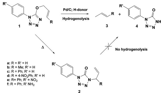
**FIGURE 1.** Hydrogenolysis and thermal isomerization of 5-allyloxy-1-aryl-tetrazoles.
