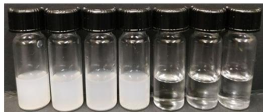
**Figure 8.** Aqueous solubility test for the tryptophan derivatives (1 mM, 20% EtOH in saline).
