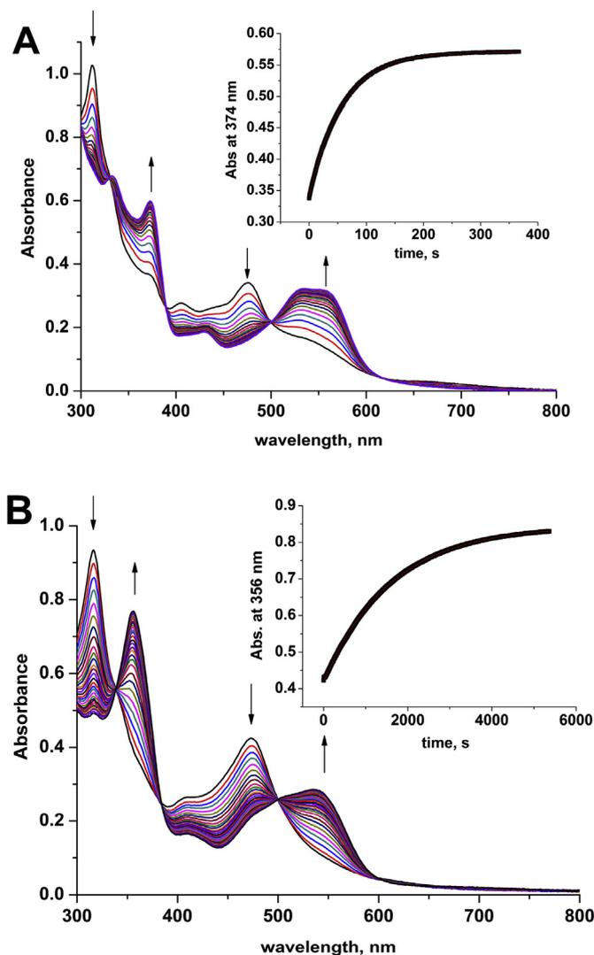
**Fig. 2.** UV/Vis spectra for the reaction between Cbl(II) ( $4 \times 10^{-5}$  M) and DHA ( $5.9 \times 10^{-4}$  M (A),  $2.7 \times 10^{-3}$  M (B)) in the presence of GSH ( $1 \times 10^{-3}$  M) at pH 5.0 (A), and  $\text{SCN}^-$  ( $1 \times 10^{-2}$  M) at pH 1.55 (B), 25 °C, and typical kinetic curves of these reactions (insets).
