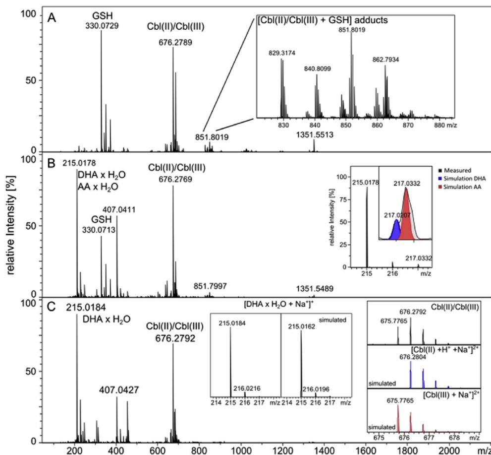
**Fig. 4.** Cryo-ESI-MS spectra of (A) mixture of Cbl(II) ( $2 \times 10^{-5}$  M) with GSH ( $10^{-4}$  M), (B) reaction mixture of Cbl(II), GSH and DHA ( $5 \times 10^{-4}$  M) and (C) mixture of Cbl(II) and DHA (without GSH).
