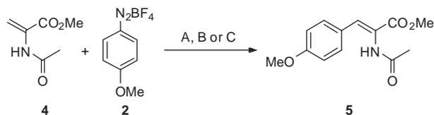
A: Pd<sub>2</sub>(dba)<sub>3</sub>, NaOAc, MeCN, 25 °C (no product detected)
