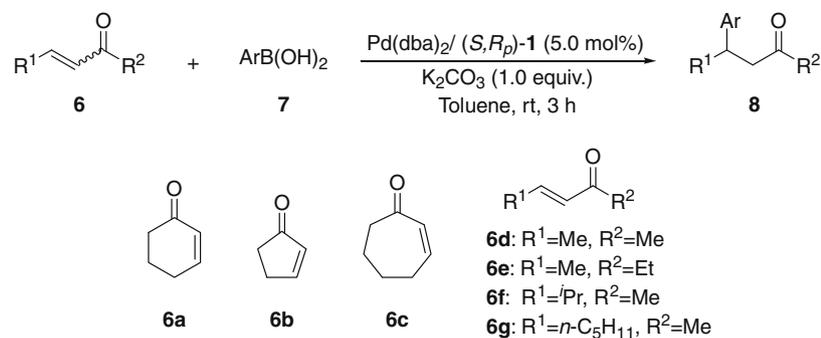
**Scheme 4.** 1,4-Addition of arylboronic acids **7** to  $\alpha,\beta$ -unsaturated ketones **6** catalyzed by palladium-(*S,R<sub>p</sub>*)-**1**.
