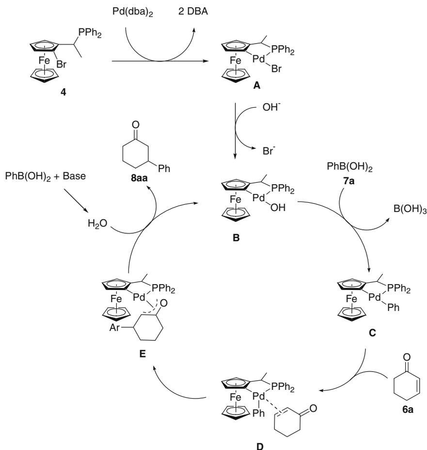
Scheme 3. Plausible reaction mechanism.
