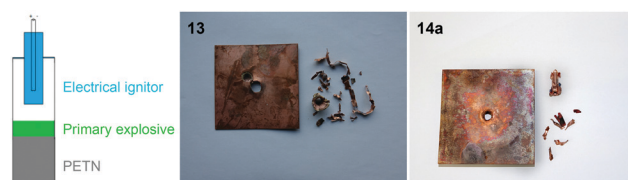
Fig. 16 Schematic setup of the PETN initiation capability test (left) as well as positive results of ECC 13 (middle) and 14a (right).
