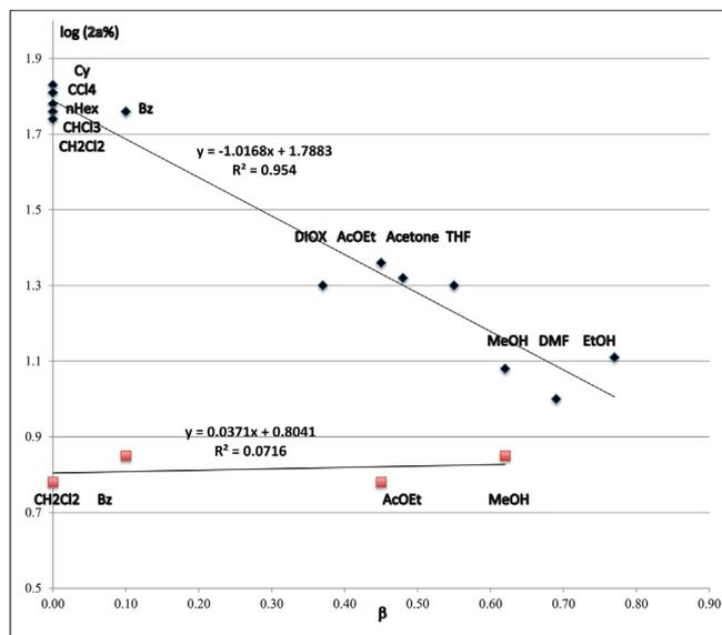
**Fig. 1.** Plot and linear regression of the log(**2a**%) vs solvents  $\beta$  values.
