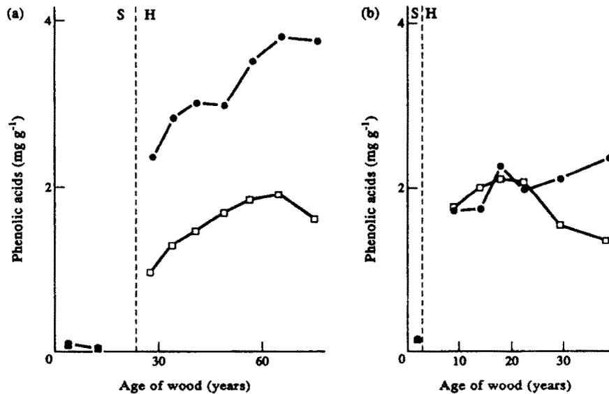
Fig. 4. Ellagic acid (●) and gallic acid (□) contents in wood radial sections of sessile oak (a) and sweet chestnut (b). S: sapwood. H: heartwood.
