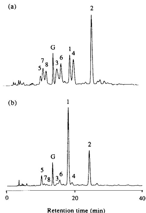
Fig. 1. Reverse-phase HPLC chromatograms of acetone-water extracts from sessile oak heartwood (a) and sweet chestnut heartwood (b). G, Gallic acid; numbers refer to the structures given in the text.
