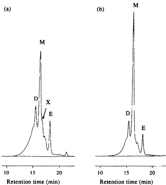
Fig. 5. Gel permeation chromatograms of acetylated extracts from sessile oak (a) and sweet chestnut (b) heartwoods. D, dimers; M, monomers; E, ellagic acid; X, tentatively assigned to vescalagin and castalin.
