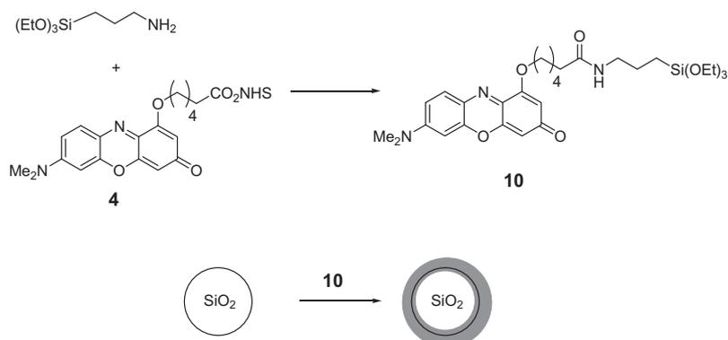
**Figure 5.** Modification of SiNPs with reactive label **4**.
