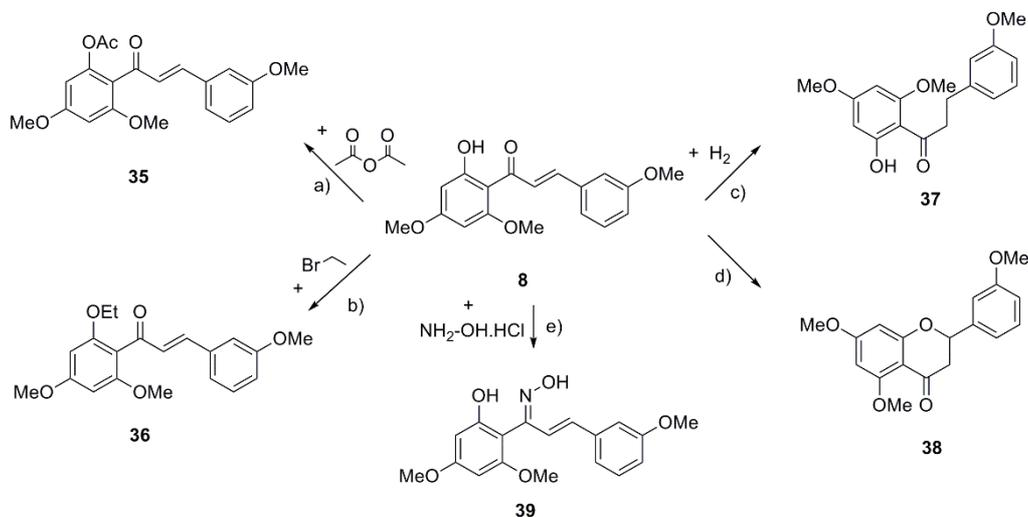
**Scheme 2.** The synthetic routes of **35** - **39**. Reagents and conditions: a) reflux; b) dry THF, NaH,  $N_2$ ,  $0^\circ C$ ; c) MeOH,  $PtO_2$ , r.t.; d) MeOH, c.c. HCl, reflux; e) MeOH, pyridine, r.t..
