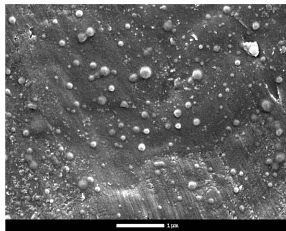
**FIGURE 7** SEM of NPs prepared from 1 mL solution of P(Glu-*oa*) 13% (3 mg/mL) with 100 μL of GCSF (4.4 mg/mL) and 60 μL of TMC (3 mg/mL).
