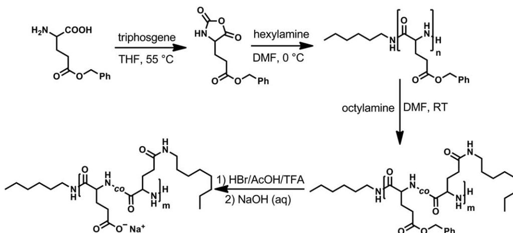
**SCHEME 1** Synthetic pathway for preparation of alkyl-modified poly(sodium glutamate)s, [P(Glu-oa)].
