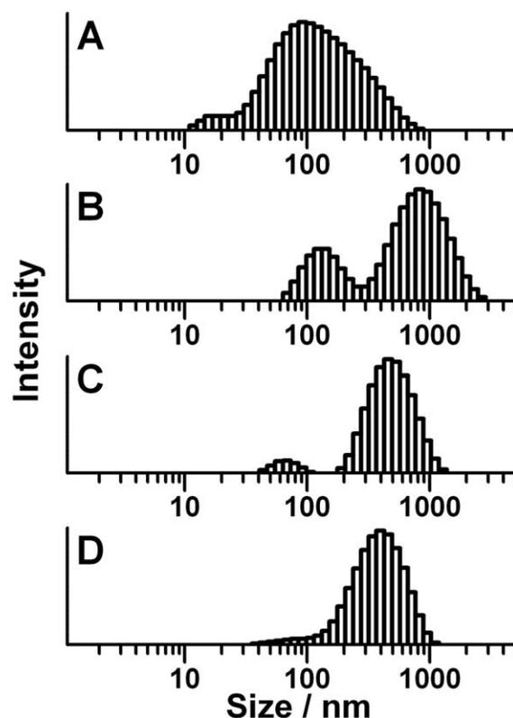
**FIGURE 6** Histograms of 1 mL solutions of P(Glu-*oa*) 13% (3 mg/mL) with 100  $\mu\text{L}$  of GCSF (4.4 mg/mL) without TMC (A) and with 10  $\mu\text{L}$  (B), 30  $\mu\text{L}$  (C), and 60  $\mu\text{L}$  (D) of TMC (3 mg/mL).
