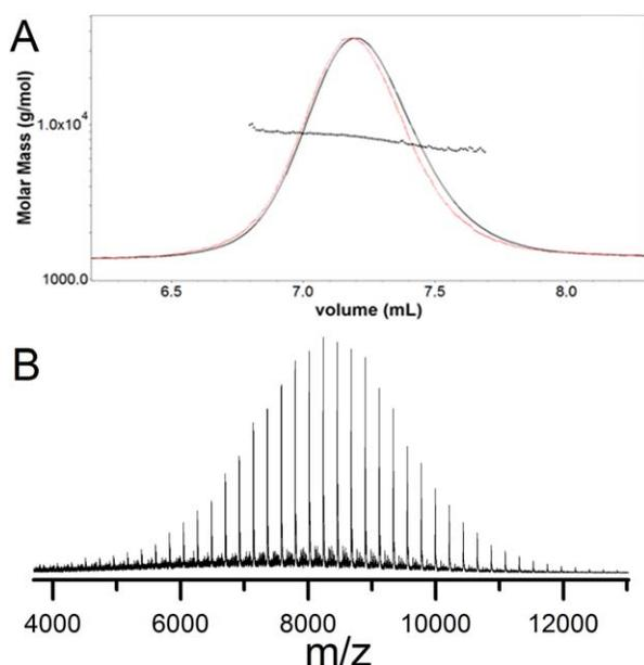
**FIGURE 1** A: SEC-MALS chromatogram of P(BLG), black solid curve: refractive index detector response, red dotted line: light-scattering detector response at 90° angle, black squares: molar mass as a function of elution volume; (B) MALDI-TOF mass spectrum of P(BLG). [Color figure can be viewed in the online issue, which is available at [wileyonlinelibrary.com](http://wileyonlinelibrary.com).]
