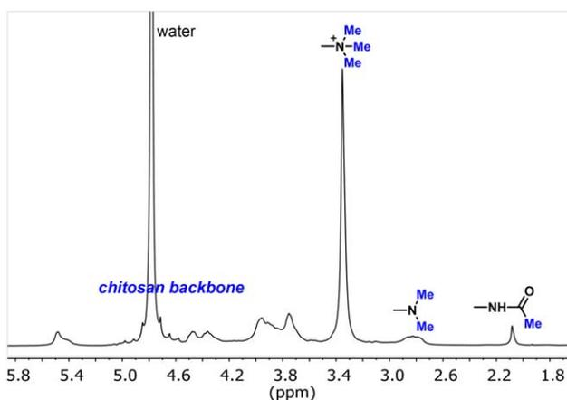
**FIGURE 5**  $^1\text{H}$  NMR spectrum of TMC with assignment of the main signals. [Color figure can be viewed in the online issue, which is available at [wileyonlinelibrary.com](http://wileyonlinelibrary.com).]
