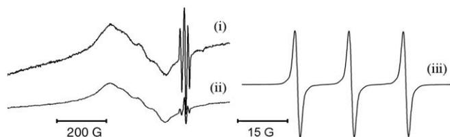
**Figure 1.** EPR spectra of (i) a THF solution prepared from  $\text{CuCl}_2\cdot\text{TMEDA}$  and  $\text{LiTMP}$  ( $2.10^{-3}$  M each), (ii) the same solution 20 h later, and (iii) a THF solution of TEMPO ( $g = 2.007$ ,  $a_N = 15.54$  G).
