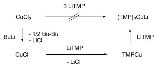
**Scheme 1.** Synthesis of  $(\text{TMP})_2\text{CuLi}$  from  $\text{CuCl}_2\cdot\text{TMEDA}$  as copper(II) source.
