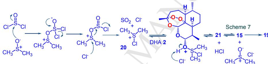
**Scheme 10.** Proposal for thionyl chloride activation by DMSO (*cf.* Scheme 7). As in the case of oxalyl chloride, the reaction is catalytic with respect to DMSO, but here  $\text{SO}_2$  rather than carbon oxides are the gaseous by-products.
