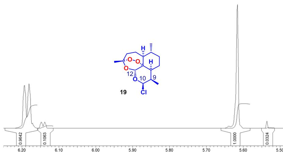
**Figure 3.** <sup>1</sup>H NMR spectrum of the  $\beta$ -chloride **19** (300 MHz, CD<sub>2</sub>Cl<sub>2</sub>). The signal due to H-12 is at  $\delta$  5.62 ppm, and H-10 is at  $\delta$  6.19 ppm; with  $J_{10,9} = 3.3$  Hz, H-10 is axial with a cis axial-equatorial coupling to H-9. Signals at  $\delta$  5.53 and 6.19 ppm are due the glycal **16**.
