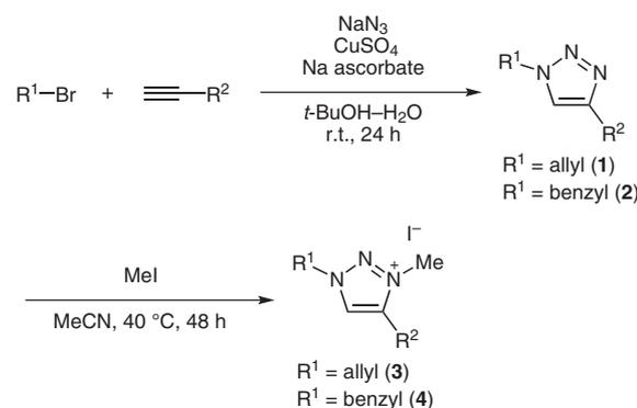
**Scheme 1** Preparation of triazoles **1** and **2** from a two-step one-pot reaction, and triazolium salts **3** and **4** from N-alkylation with methyl iodide
