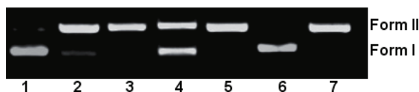
Fig. 5. Gel electrophoresis showing the chemical nuclease activity of CT-DNA incubated at 37 °C for 2 h with different concentrations of complexes 1–3; lane 1, DNA control; lane 2, DNA + complex 1 (30 μM); lane 3, DNA + complex 1 (60 μM); lane 4, DNA + complex 2 (30 μM); lane 5, DNA + complex 2 (60 μM); lane 6, DNA + complex 3 (30 μM); lane 7, DNA + complex 3 (60 μM).
