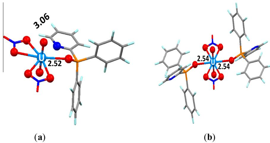
**Fig. 3.** (a) Optimized structures for  $[UO_2(NO_3)_2L]$  and (b)  $[UO_2(NO_3)_2 \cdot 2L]$ .
