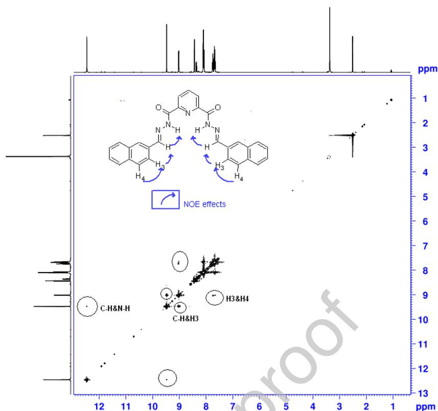
**Figure 2.** 2D NOESY of **3f** in DMSO-*d*<sub>6</sub> at 295 K (x- and y-axis, <sup>1</sup>H-NMR chemical shift).
