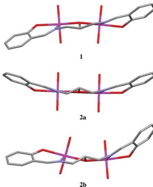
**Fig. 4** Distortion observed in the backbone of **1**·(DMF)<sub>2</sub>, **2a** and **2b**. The *tert*-butyl groups in **2a** and **2b** are omitted for clarity.<sup>45</sup>
