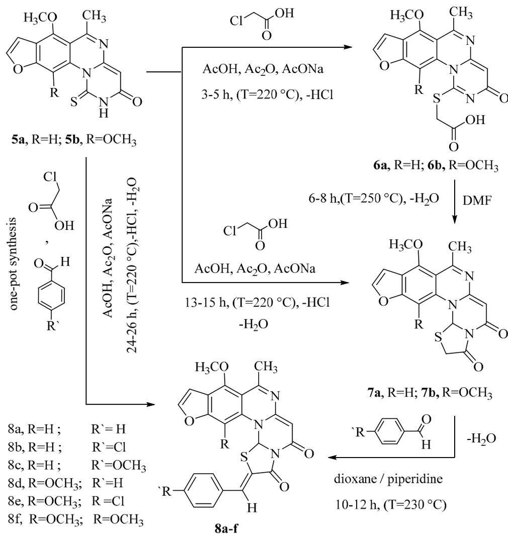
**Scheme 2.** Synthesis of furothiazolopyrimidoquinazolinone derivatives.
