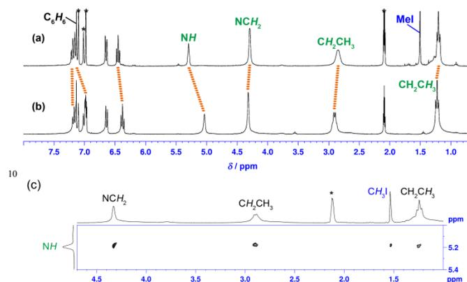
**Fig. 1**  $^1\text{H}$  NMR spectra (300 MHz, 298 K, toluene- $d_8$  (\*)) of MeI@**1** (a) purified **1** (b). (c) partial  $^1\text{H}$ - $^1\text{H}$  NOESY spectrum of MeI@**1**.
