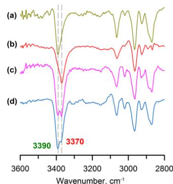
**Fig. 2** Partial solid-state IR spectra of **1** as synthesized (a), crystalline  $\text{I}_2$ @**1** (b), crystalline MeI@**1** (c), and soild MeI@**1** after exposure to the atmosphere for over 24 h under ambient conditions (d). The dashed gray lines represent the N-H stretching frequencies at 3370 and 3390  $\text{cm}^{-1}$ .
