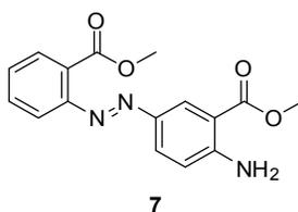
**Figure 5.** Structure of azo-coupling by-product.
