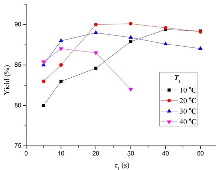
**Figure 6.** Effect of diazotization reaction temperature and residence time on the yield.
