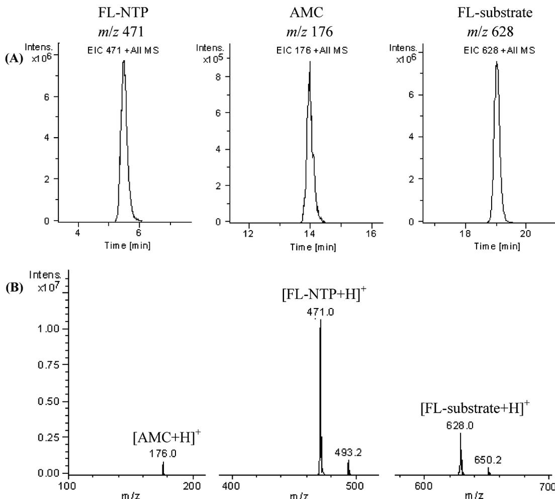
**Figure 2.** LC chromatograms and mass spectra for the FL-substrate and its products, FL-NTP and AMC. (A) Extracted ion chromatogram (EIC) of FL-NTP ( $m/z$  471), AMC ( $m/z$  176), and FL-substrate ( $m/z$  628). (B) Mass spectra of FL-NTP, AMC, and FL-substrate in full scan mode from  $m/z$  100 to 700. Peaks at  $m/z$  493 and 650 are  $\text{Na}^+$  adducts and were not quantified.
