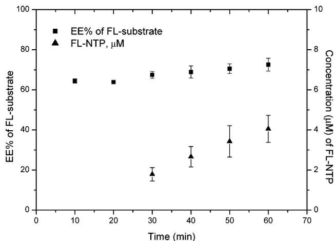
**Figure 4.** Time-dependent delivery of FL-substrate and FL-NTP recovery during single-substrate dialysis. FL-substrate (50  $\mu\text{M}$ ) was perfused at 1  $\mu\text{L}/\text{min}$  to a quiescent solution containing 0.5 units/mL elastase at 37  $^{\circ}\text{C}$ . FL-NTP concentrations in the 10 and 20 min dialysate samples were below the LOQ. Symbols and error bars denote mean  $\pm$  SD,  $n = 3$ .
