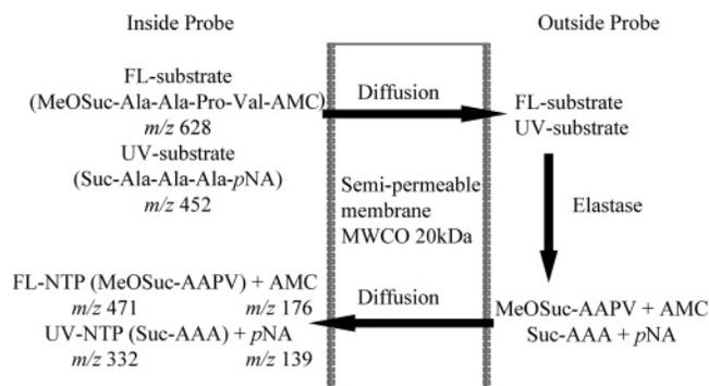
**Figure 1.** Microdialysis sampling schematic. FL-substrate and UV-substrate diffuse to the surrounding medium react with elastase forming products that diffuse back into the probe.
