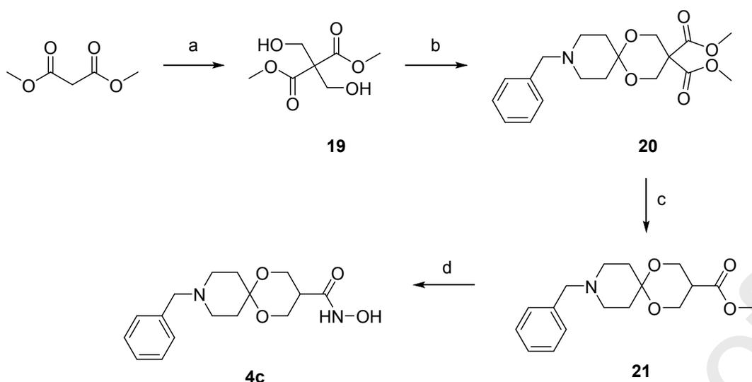
**Scheme 2.** Reagents and conditions: (a) 30% aq. formaldehyde (3 equiv.), saturated solution of NaHCO<sub>3</sub>, r.t., overnight, 30% yield; (b) 4-benzyl-piperidone (0.75 equiv.), *p*TSA (cat.), N<sub>2</sub>, Dean-Stark trap, 24 h, 48% yield; (c) NaCl (1.2 equiv.), DMSO, 180 °C, 4 h, 87% yield; (d) 50% aq. NH<sub>2</sub>OH, EtOH, r.t., 24 h, 12% yield.
