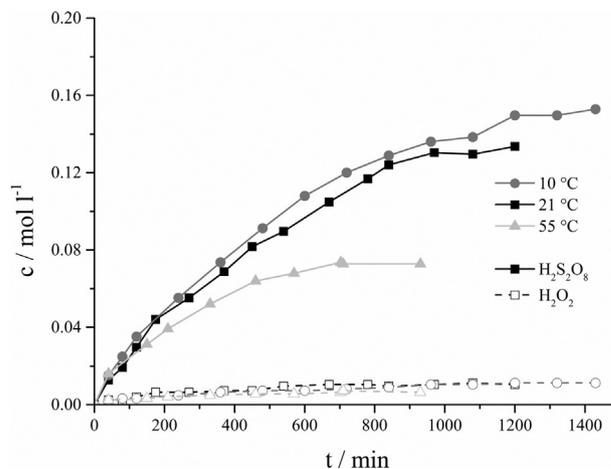
**Fig. 5.** Concentrations of H<sub>2</sub>S<sub>2</sub>O<sub>8</sub> and H<sub>2</sub>O<sub>2</sub> vs. time in sulfuric acid (90 wt%) using three different working temperatures, current density = 0.15 A cm<sup>-2</sup>.
