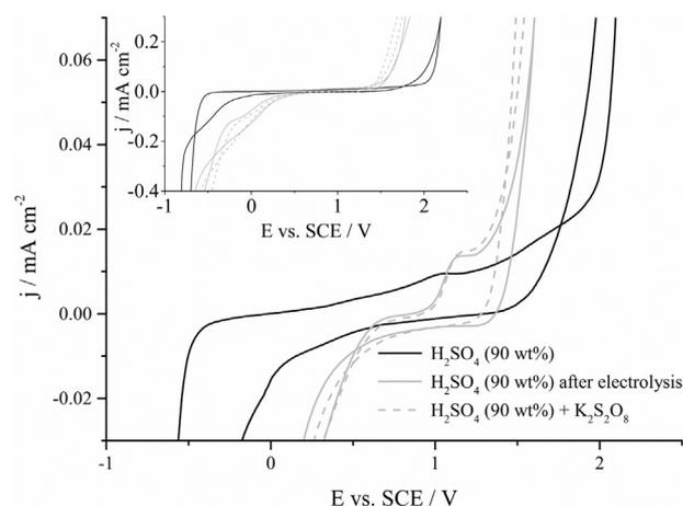
Fig. 4. Cyclic voltammogram of boron-doped diamond electrodes in H<sub>2</sub>SO<sub>4</sub> (90 wt%), before and after electrolysis, and after addition of K<sub>2</sub>S<sub>2</sub>O<sub>8</sub>, scan rate = 50 mV s<sup>-1</sup>, T = 21  $^{\circ}\text{C}$ , reference electrode SCE, counter electrode platinum, lower magnification in the inset.
