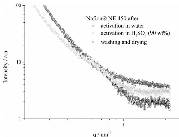
Fig. 9. Small angle X-ray scattering curves of Nafion NE 450 membranes after different activation procedures at room temperature.
