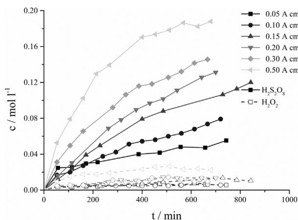
Fig. 7. Concentrations of  $\text{H}_2\text{S}_2\text{O}_8$  species and  $\text{H}_2\text{O}_2$  vs. time in sulfuric acid (90 wt%), constant temperature ( $21^\circ\text{C}$ ) using six different current densities.
