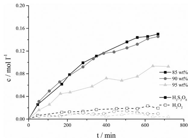
Fig. 8. Concentrations of  $\text{H}_2\text{S}_2\text{O}_8$  and  $\text{H}_2\text{O}_2$  vs. time at constant temperature ( $21^\circ\text{C}$ ), constant current ( $0.15 \text{ A cm}^{-2}$ ) using three different  $\text{H}_2\text{SO}_4$  concentrations.
