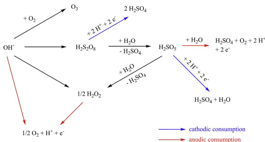
Fig. 6. Possible reaction paths of hydroxyl radicals after desorption, including anodic and cathodic consumption reactions.
