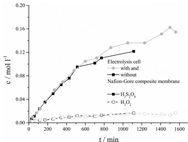
Fig. 10. Concentrations of  $\text{H}_2\text{S}_2\text{O}_8$  and  $\text{H}_2\text{O}_2$  vs. time in sulfuric acid (90 wt%), current density =  $0.15 \text{ A cm}^{-2}$  for electrolysis cell with and without Nafion-Gore composite membrane.
