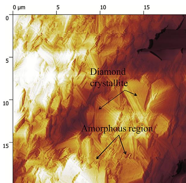
Fig. 2. Atomic force microscopy of the BDD electrode surface scanned in tapping mode with a resonance frequency of 150 kHz.
