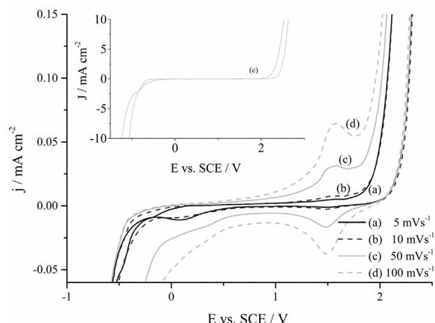
Fig. 3. Cyclic voltammogram of boron-doped diamond electrodes in 1 M H<sub>2</sub>SO<sub>4</sub> at different scan rates, T = 21  $^{\circ}\text{C}$ , reference electrode SCE, counter electrode platinum, lower magnification in the inset.
