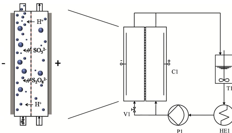
**Fig. 1.** Schematic description of the modified electrolyte cell with two half cells separated by a manufactured Nafion membrane (left) and technical drawing of the setup used for electrolysis of  $\text{H}_2\text{SO}_4$  on BDD (right); C1 electrolytic flow cell, P1 PTFE membrane pump, HE1 PFA heat exchanger, V1 valve, T1 electrolyte reservoir.
