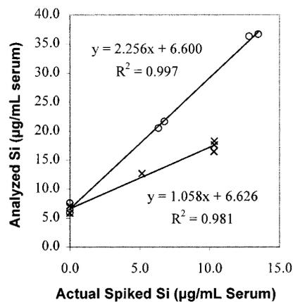
Figure 1. ICP-AES analysis of sample prepared by microwave digestion of poly(dimethylsiloxane)-spiked pig serum in HNO<sub>3</sub>. ○ – poly(dimethylsiloxane)-spiked serum, x – silicate-spiked serum.
