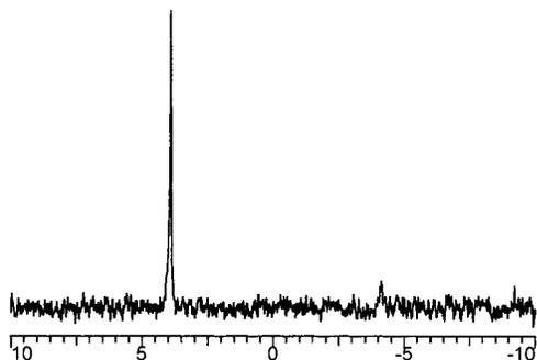
Figure 2.  $^{29}\text{Si}$  NMR spectrum of a 0.0312% solution of  $(\text{CH}_3)_2\text{Si}(\text{OH})_2$  in pig serum. Spectrum was acquired with 256 scans in 17.1 h. Peak at 3.9 ppm is dimethylsilanediol,  $s/n = 34.6$ . The peak at  $-4.2$  ppm arises from trace levels of the condensation product, tetramethyldisiloxanediol.
