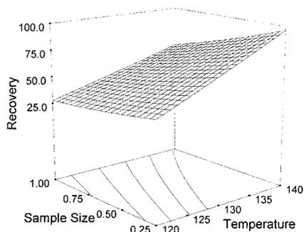
Figure 3. Response surface for recovery as a function of sample size and temperature during microwave digestion of poly(dimethylsiloxane)-spiked pig serum in 10 wt. % HCl.
