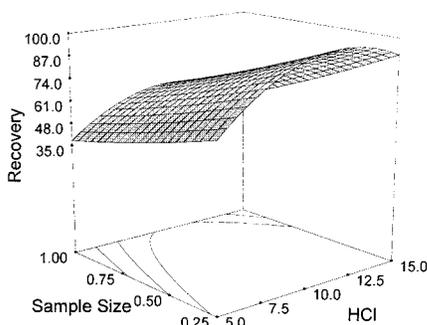
Figure 4. Response surface for recovery as a function of sample size and HCl concentration during microwave digestion of poly(dimethylsiloxane)-spiked pig serum at 140 °C.
