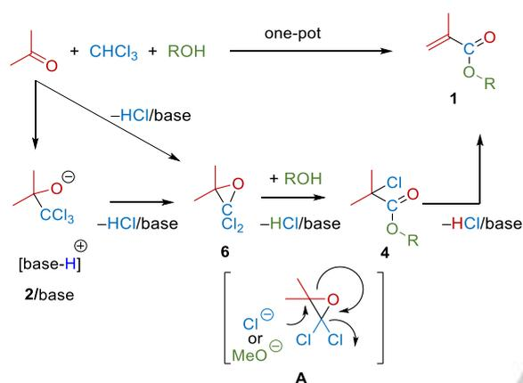
**Scheme 2.** Possible reaction mechanism for the one-pot formation of methacrylic ester in this study.
