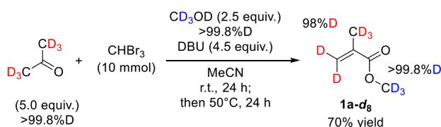
**Scheme 3.** Synthesis of deuterated MMA (**1a-d<sub>8</sub>**)
