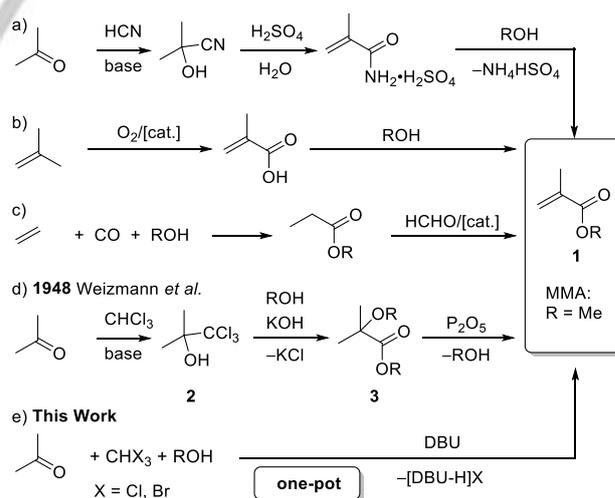
**Scheme 1.** Synthetic methods of methacrylates: Current industrial processes for MMA synthesis (a–c) versus the route from acetone, chloroform, and alcohols (d and e).
