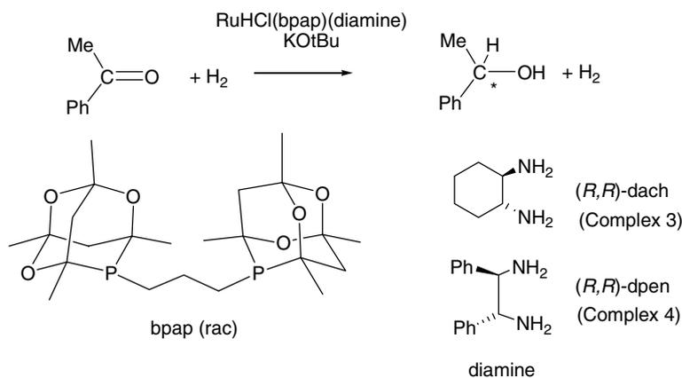
Fig. 5. Hydrogenation (3 atm H<sub>2</sub>) of acetophenone catalyzed by complexes **3** and **4** in neat ketone at 20 °C.
