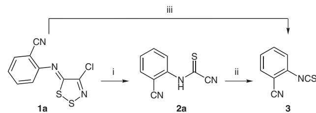
**Scheme 1** Reagents and conditions: (i) DBU (3 equiv), CH<sub>2</sub>Cl<sub>2</sub>, -5 °C, 5 min, 93%; (ii) DBU (1 equiv), 20 °C, 0.5 h, 95%; (iii) DBU (4 equiv), CH<sub>2</sub>Cl<sub>2</sub>, -5 to +20 °C, 0.5 h, 96%.
