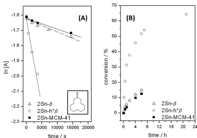
Fig. 10 (A) Initial rate data for 2Sn- $\beta$  (open triangles), 2Sn-h\* $\beta$  (open circles) and 2Sn-MCM-41 (filled squares) for the MPV reduction of cyclododecanone, and (B) extended time online profile for the same reactions.
