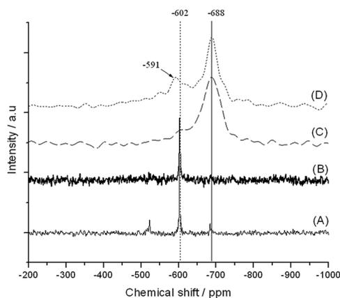
Fig. 6 MAS NMR spectra of (A) SnO<sub>2</sub>, (B) 10% SnO<sub>2</sub>/deAl- $\beta$  (physical mixture), (C) 2Sn- $\beta$ , and (D) 2Sn-h\* $\beta$ .
