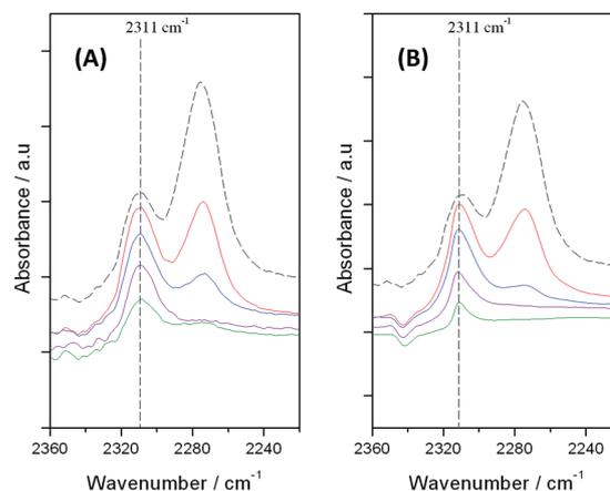
Fig. 5 *In situ* DRIFTS spectra of (A) 2Sn-h\* $\beta$ , and (B) 2Sn- $\beta$ , following (dashed) 10 minute treatment with CD<sub>3</sub>CN at room temperature. Various desorption temperatures (50 (red), 100 (blue), 150 (purple) and 200 °C (green)) are also displayed.
