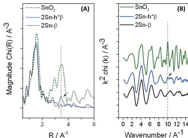
Fig. 7 (A) Magnitude of the Fourier transform spectra, and (B) EXAFS  $k^3$ -weighted  $x$  data, of 2Sn- $\beta$ , (black) and 2Sn-h\* $\beta$  (blue). The corresponding spectra of SnO<sub>2</sub> (green dots) are also displayed.
