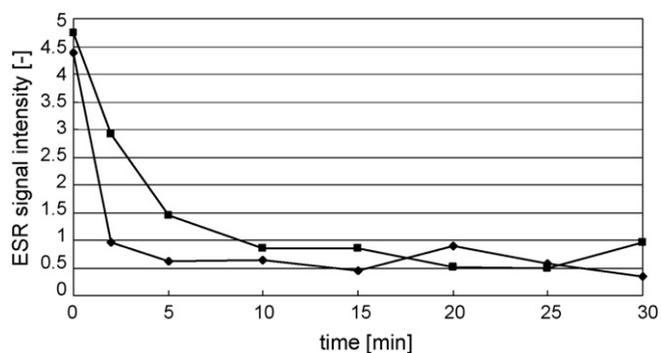
**Fig. 9.** Time-course of the decay in ESR intensity after addition of 15-mM PBS solution of Na ascorbate to 20-μM PBS solutions of 3-amino-PROXYL (**6**, ♦) and **21** (■) (1:1, v/v), respectively.
