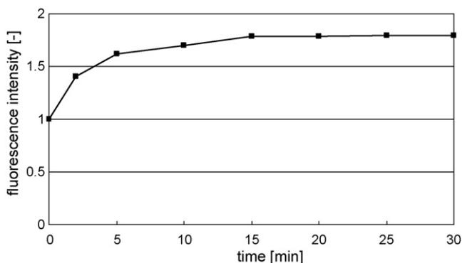
**Fig. 10.** Time-course of the increase in fluorescence intensity ( $0.2 \mu\text{M}$ ,  $\lambda_{\text{ex}}$  620 nm) after addition of a 15-mM PBS solution of Na ascorbate to a 20-mM PBS solution of **21** (1:1, v/v).
