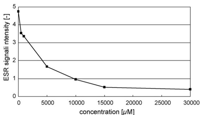
**Fig. 11.** ESR intensity at 20 min after the addition of various concentrations of a PBS solution of Na ascorbate to a 20- $\mu\text{M}$  PBS solution of **21** (1:1, v/v).
