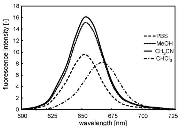
Fig. 6. Fluorescence intensity of Cy5 (**8**) in some solvents ( $c$  0.2  $\mu$ M,  $\lambda_{\text{ex}}$  = 630 nm).
