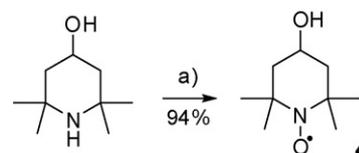
**Scheme 3.** Synthesis of 4-hydroxy-TEMPO (**6**). Reagents and conditions: (a) 30%  $\text{H}_2\text{O}_2$ , EDTA,  $\text{Na}_2\text{WO}_4$ , in  $\text{H}_2\text{O}$ , r.t. 1 day.
