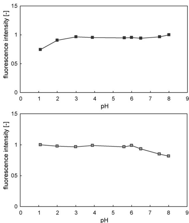
**Fig. 8.** Effect of pH on the fluorescence intensity of **8** (1.0 μM, upper panel) and **21** (1.0 μM, lower panel).
