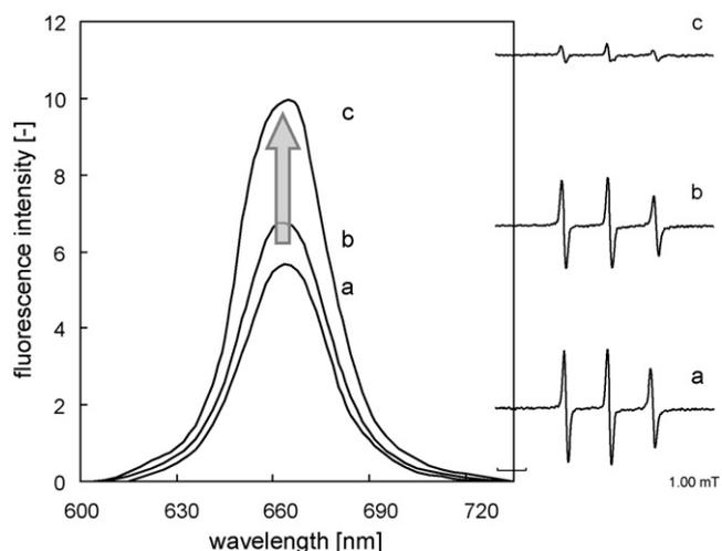
Fig. 7. Changes in fluorescence ( $\lambda_{\text{ex}}$  649 nm) and ESR spectra at 20 min after three concentrations of Na ascorbate in PBS (a: 0 mM, b: 1.0 mM, c: 30 mM) were added to a 20- $\mu$ M solution of **21** in PBS (pH 7.0) (1:9, v/v).
