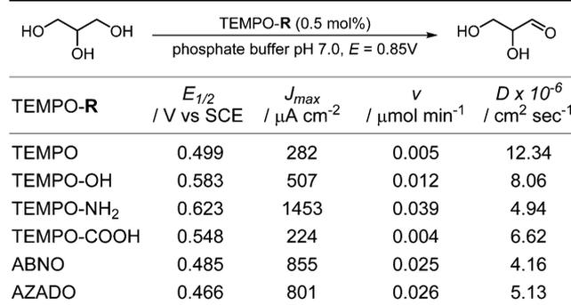
**Figure 1.** Electrocatalytic screening of TEMPO compounds with glycerol. Catalytic activity was determined by comparison of cyclic voltammograms in the presence and absence of 0.1 M glycerol using 40 mM Robinson buffer, pH = 7.0, at 25 °C.
