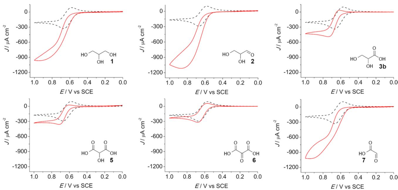
**Figure 3.** Catalytic CVs of 5 mM TEMPO-NH<sub>2</sub> in the absence (dashed) and presence (solid) of 100 mM substrate: (left to right, top row) glycerol, glycerinaldehyde, glyceric acid, (second row) tartronic acid, mesoxalic acid, glyoxylic acid. Experiments were performed using a 3 mm glassy carbon electrode with 50 mM phosphate buffer, pH 5.2, at 5 mV s<sup>-1</sup> and 25 °C.
