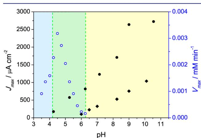
**Figure 2.** Overlaid pH profiles of oxalate oxidase (○), TEMPO (◆), and TEMPO-NH<sub>2</sub> (●). Dotted lines highlight the overlapping pH range between OxO and TEMPO-NH<sub>2</sub>.
