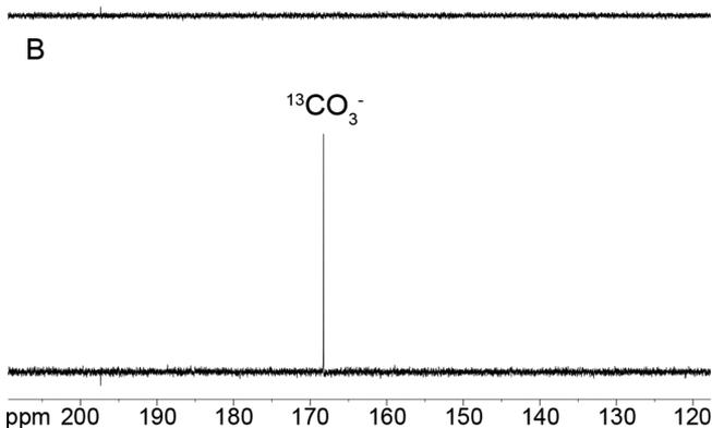
**Figure 4.**  $^{13}\text{C}$  NMR spectrum of (a) a control sample of NaOH exposed to ambient conditions for 22 h, and (b)  $^{13}\text{CO}_2$  trapped in the form of  $\text{Na}_2{}^{13}\text{CO}_3$  from  $^{13}\text{C}$ -labeled glycerol that was completely oxidized from a solution of TEMPO-NH<sub>2</sub> and OxO.
