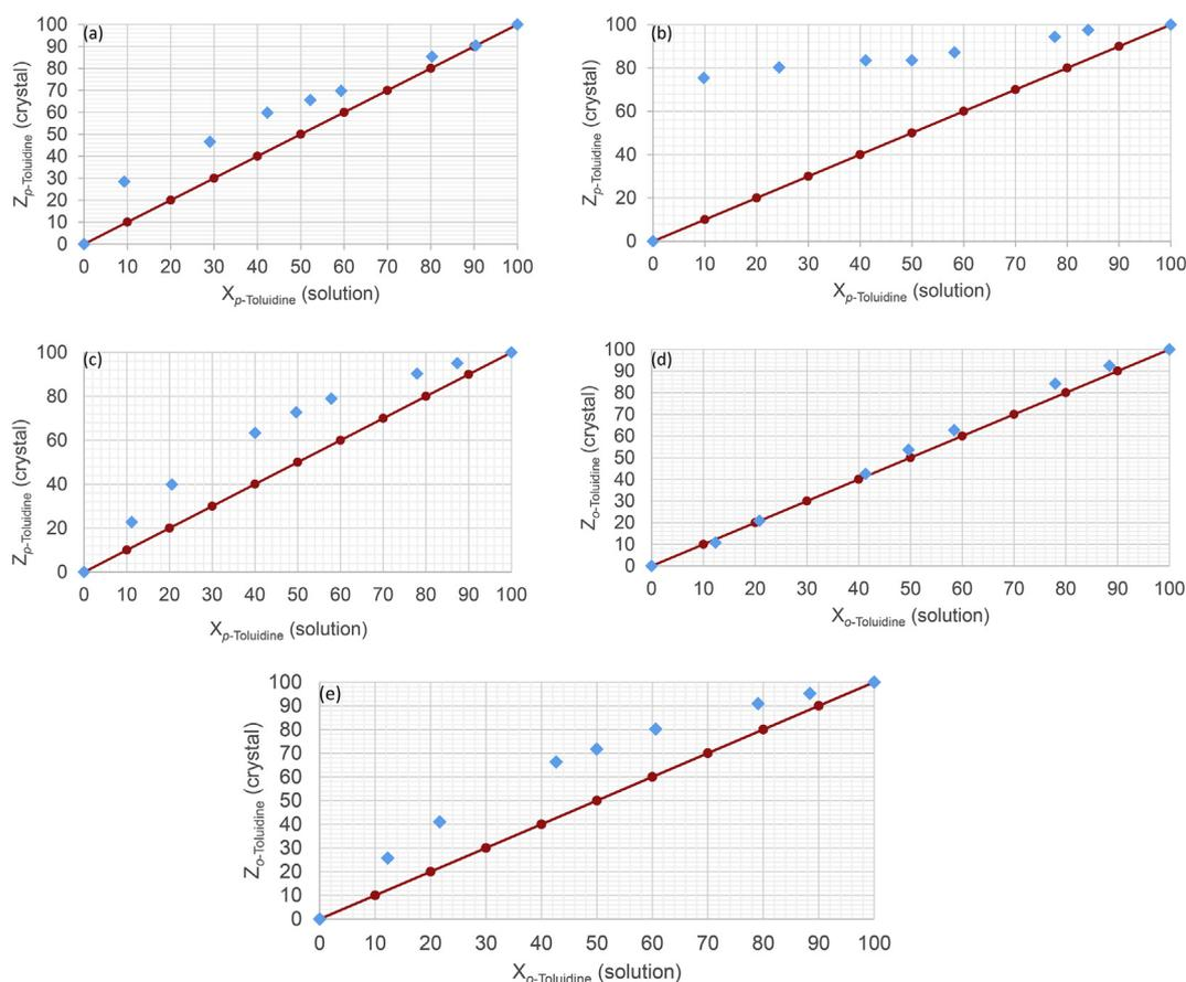
Fig. 1. Selectivity profiles for (a) **TETROL**/*p*-TOL/*m*-TOL, (b) **TETROL**/*p*-TOL/*o*-TOL, (c) **DMT**/*p*-TOL/*m*-TOL, (d) **DMT**/*p*-TOL/*o*-TOL and (e) **DMT**/*o*-TOL/*m*-TOL experiments.
