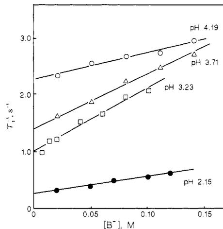
**Figure 3.** Buffer catalysis of the τ<sub>1</sub><sup>-1</sup> process in the pH-jump experiments with the morpholine adduct: open symbols, chloroacetate buffer; filled symbols, dichloroacetate buffer. Data from Table S3.
