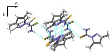
**Figure 3** Formation of N(6)···S(2) H-bonded centrosymmetric layers and a cavity down the *c* axis.
