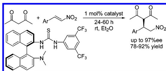
A novel binaphthyl-derived amine thiourea organocatalyst has been developed and demonstrated to efficiently catalyze Michael addition reactions (using as low as 1 mol % loading) of diketones to nitroalkenes with remarkably high enantioselectivities.
