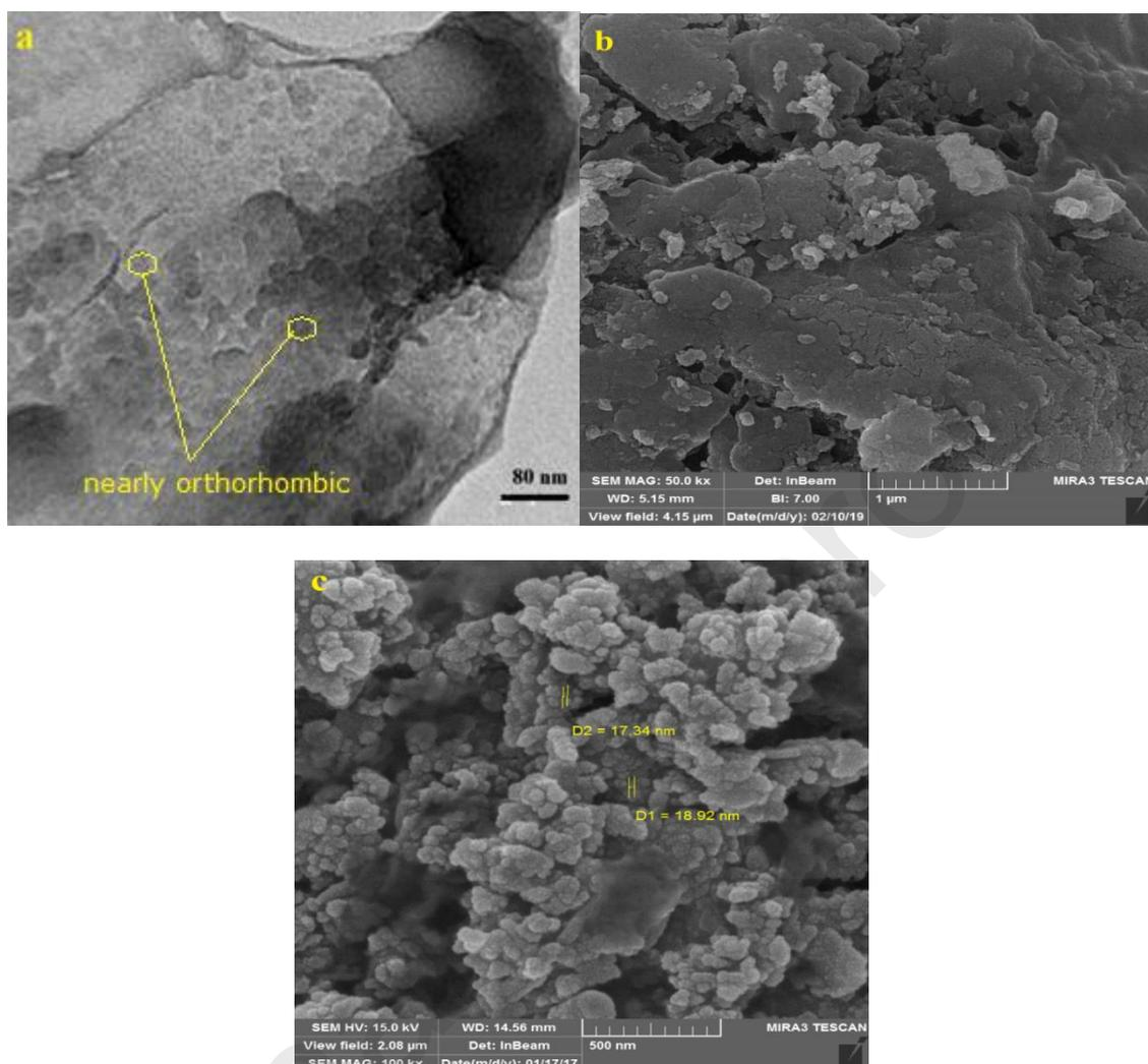
**Fig. 4.** a) TEM image of BNP@SiO<sub>2</sub>(CH<sub>2</sub>)<sub>3</sub>NH<sub>3</sub>SO<sub>3</sub>H, b) SEM image of boehmite and c) SEM image of the BNP@SiO<sub>2</sub>(CH<sub>2</sub>)<sub>3</sub>NH<sub>3</sub>SO<sub>3</sub>H
