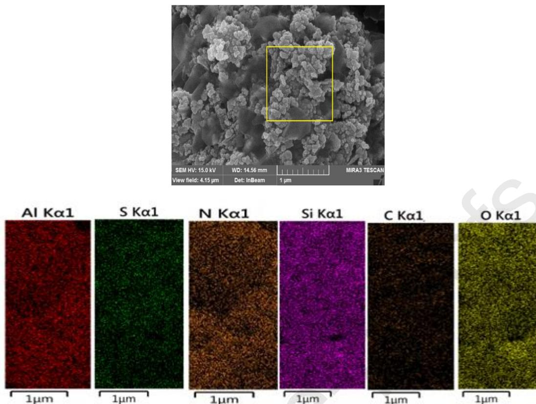
**Fig. 7.** Mapping pattern of the BNPs@SiO<sub>2</sub>(CH<sub>2</sub>)<sub>3</sub>NHSO<sub>3</sub>H
