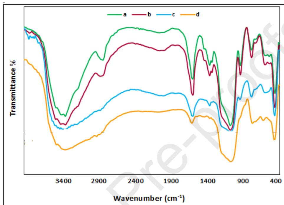
**Fig. 3.** FTIR spectra of a) BNPs, b) BNPs-TEOS, c)  $\text{BNPs}@SiO_2(\text{CH}_2)_3\text{NH}_2$  and d)  $\text{BNPs}@SiO_2(\text{CH}_2)_3\text{NHSO}_3\text{H}$
