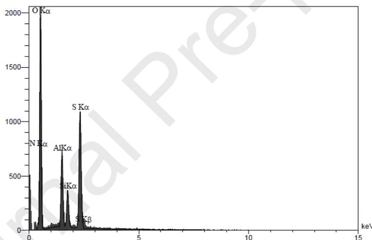
**Fig. 6.** EDX spectrum of the nano-catalyst
