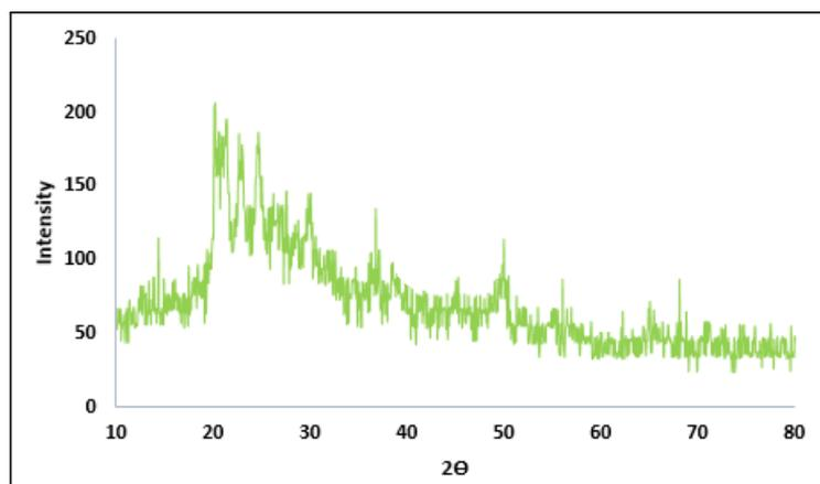
**Fig. 5.** XRD pattern of BNPs@SiO<sub>2</sub>(CH<sub>2</sub>)<sub>3</sub>NHSO<sub>3</sub>H
