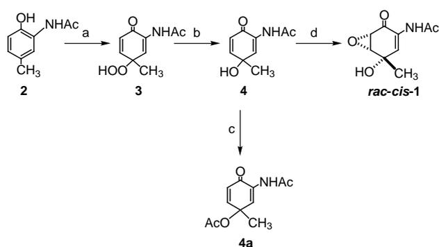
**Scheme 2** Reagents: (a) O<sub>2</sub>, TPP, hv, acetone/CH<sub>2</sub>Cl<sub>2</sub>, –25 °C, 2 d, 62% yield; (b) Me<sub>2</sub>S (1.2 equiv), Ti(O-*i*-Pr)<sub>4</sub> (5 mol%), CH<sub>2</sub>Cl<sub>2</sub>, 20 °C, 1 h, 4 Å molecular sieves, 83% yield; (c) Ac<sub>2</sub>O, pyridine, CH<sub>2</sub>Cl<sub>2</sub>, 20 °C, 5 d, 67% yield (relative to converted material, conversion ca. 60%); (d) TBHP (1.2 equiv), DBU, CH<sub>2</sub>Cl<sub>2</sub>, 20 °C, 3 d, 78% yield.
