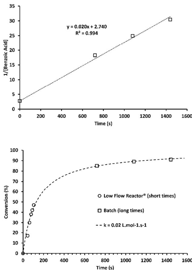
**Figure 3.** Kinetics of benzoic acid alkylation by  $\text{CH}_3\text{I}$  in the presence of DBU in a batch reactor. Second order kinetic treatment (upper panel). Batch (long times) and Low Flow (short times) superimposition (bottom panel).
