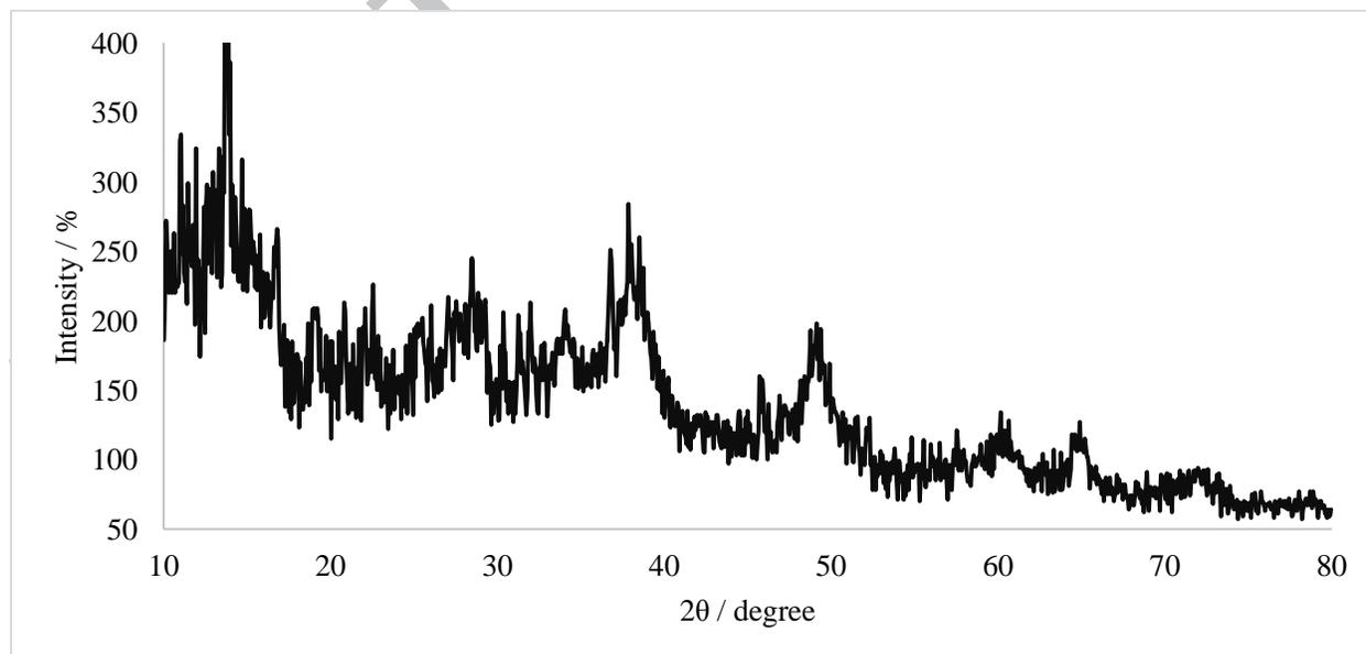
**Figure 2.** XRD pattern of Cu-Adenine@boehmite.
