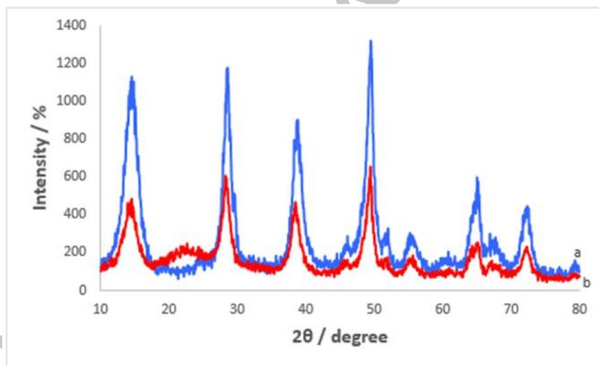
**Fig 5.** The XRD pattern of boehmite nanoparticles (a) and Cu-Adenine@boehmite after recycling (b).
