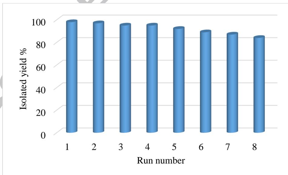
**Fig 4.** Recyclability of Cu-Adenine@boehmite in the coupling of iodobenzene (1 mmol) with PhB(OH)<sub>2</sub> (1 mmol).
