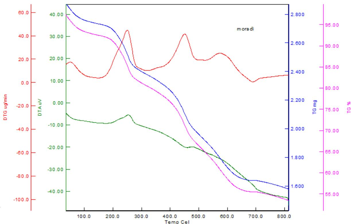
**Figure 3.** TGA/DTA diagrams of Cu-Adenine@boehmite.
