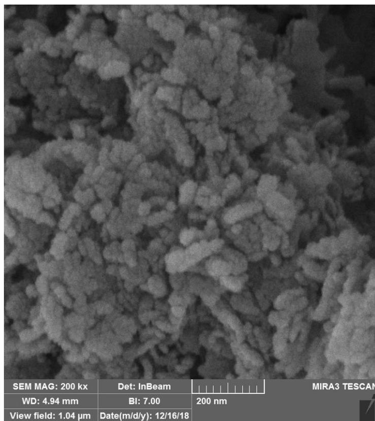
**Fig 6.** SEM image of Cu-Adenine@boehmite after recycling.
