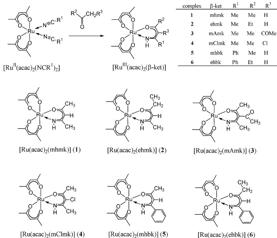
Fig. 1. The formation reactions of the  $\beta$ -ketiminato ruthenium(III) complexes and their structural formulas.
