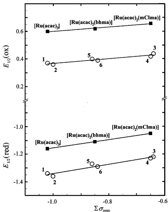
Fig. 7. Dependence of  $E_{1/2}$  on  $\sum\sigma_{\text{pmmp}}$ .  $\sum\sigma_{\text{pmmp}}$  is the sum of Hammett substituent constants [19,20] on  $\beta$ -ketiminate ( $\circ$ ) or  $\beta$ -diketonate ( $\blacksquare$ ). Slope ( $\beta$ -ketiminate): oxidation;  $0.18 \text{ V}$ , reduction  $0.34 \text{ V}$ . Slope ( $\beta$ -diketonato): oxidation;  $0.16 \text{ V}$ , reduction;  $0.30 \text{ V}$ .
