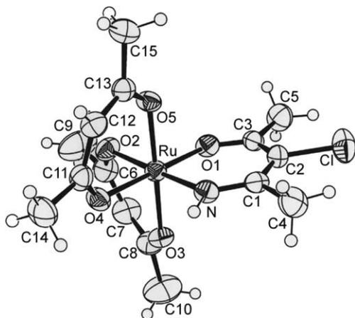
Fig. 4. Molecular structure of [Ru(acac)<sub>2</sub>(mClmk)] (4).
