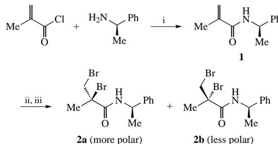
**Scheme 1** Reagents and conditions: i, Et<sub>3</sub>N, CH<sub>2</sub>Cl<sub>2</sub>, 0 → 20 °C, 4 h, 83%; ii, Br<sub>2</sub>, CH<sub>2</sub>Cl<sub>2</sub>, room temperature, 1 h, 73%; iii, SiO<sub>2</sub>, column chromatography.
