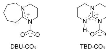
Scheme 1. The structures of the hypothetical DBU–CO<sub>2</sub> zwitterionic adduct and the proven and isolated TBD–CO<sub>2</sub> adduct.
