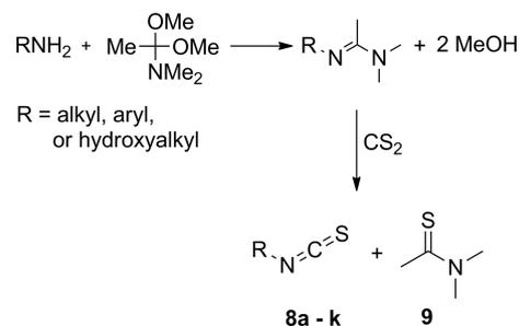
Scheme 9. The preparation of *N,N*-dimethylacetamidines and their reaction with CS<sub>2</sub>.
