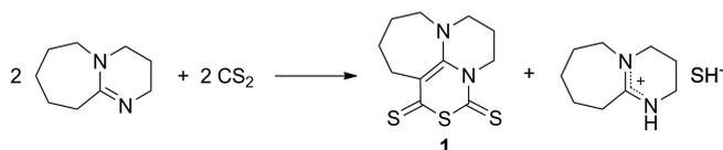
Scheme 2. The reaction of DBU with CS<sub>2</sub>.<sup>[24]</sup>
