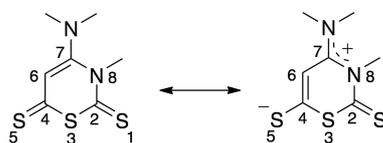
Scheme 6. Two resonance forms for the cores of compounds **1**, **3**, and **5**.
