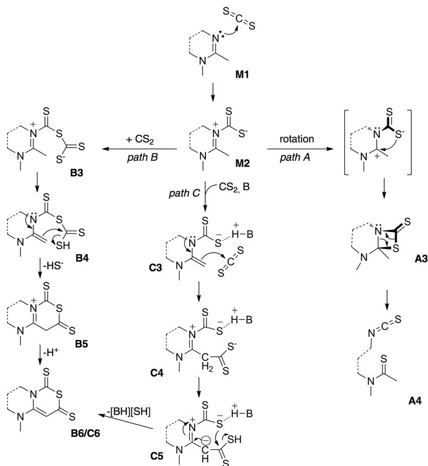
Scheme 10. Proposed mechanisms for the reaction of CS<sub>2</sub> with cyclic or acyclic amidines. Path A is analogous to Barton's mechanism<sup>[47]</sup> for the reaction of guanidines. The Vlasse mechanism<sup>[24]</sup> for DBU is path B. Our proposed mechanism for cyclic amidines is path C.
