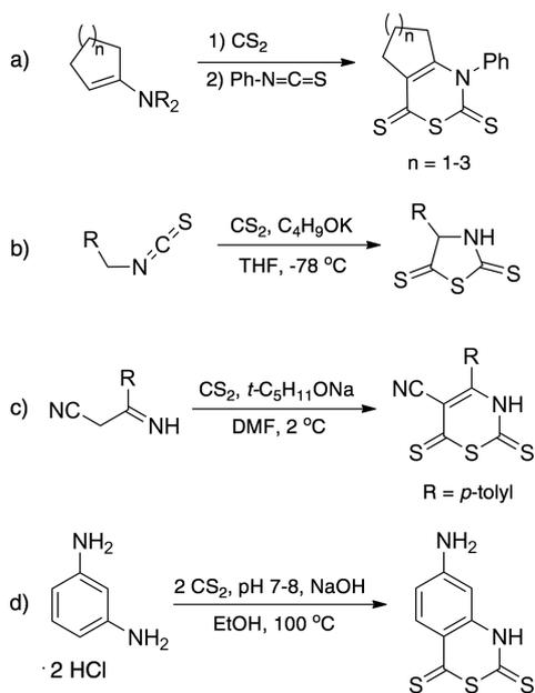
Scheme 3. Literature methods for the formation of carbamic carboxylic trithioanhydride rings: a) with CS<sub>2</sub> and phenylisothiocyanate;<sup>[25,26]</sup> b) 4-arylthiazolidene-2,5-dithiones<sup>[27]</sup> and c) 1,3-thiazine-2,6-dithiones;<sup>[28]</sup> d) from diaminobenzene and CS<sub>2</sub>.<sup>[29]</sup>
