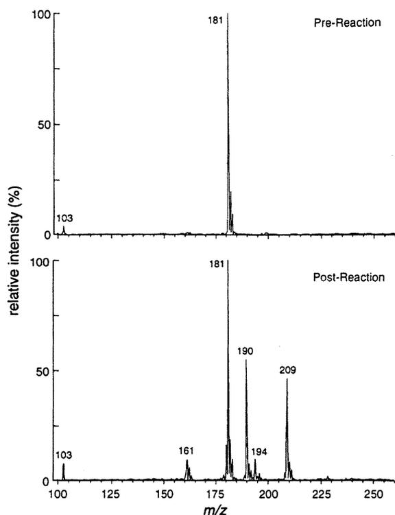
Fig. 3 API MS spectra before and after irradiation of a  $\text{Cl}_2$ - $[\text{H}_2^{18}\text{H}_8]$ hexamethyldisiloxane-air mixture
