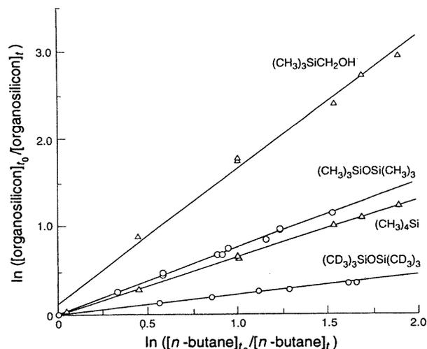
**Fig. 1** Plots of eqn. (1) for the gas-phase reactions of the Cl atom with hexamethyldisiloxane, [ $^2\text{H}_{18}$ ]hexamethyldisiloxane, tetramethylsilane and trimethylsilylmethanol, with *n*-butane as the reference compound
