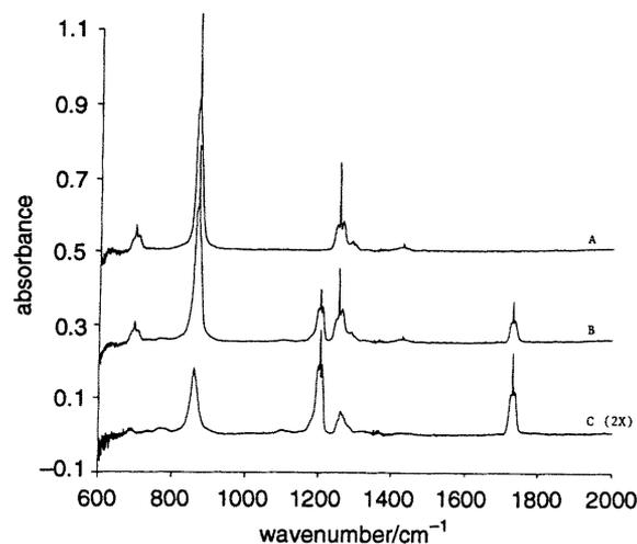
Fig. 8 IR spectra from the photolysis of a  $\text{Cl}_2$ -tetramethylsilane-air mixture. A, Initial tetramethylsilane ( $7.2 \times 10^{13}$  molecule  $\text{cm}^{-3}$ ). B, Reaction mixture after 7 min of irradiation (25% reaction). C, From B after subtraction of unreacted tetramethylsilane. The ordinates of the upper plots are offset for clarity.
