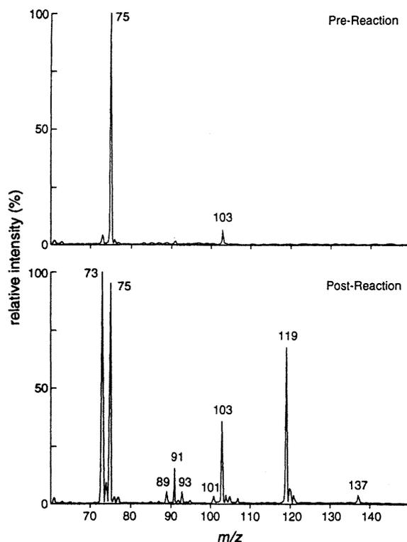
Fig. 6 API MS spectra of a  $\text{Cl}_2$ -tetramethylsilane-air mixture before (top) and after (bottom) irradiation for 2.0 min
