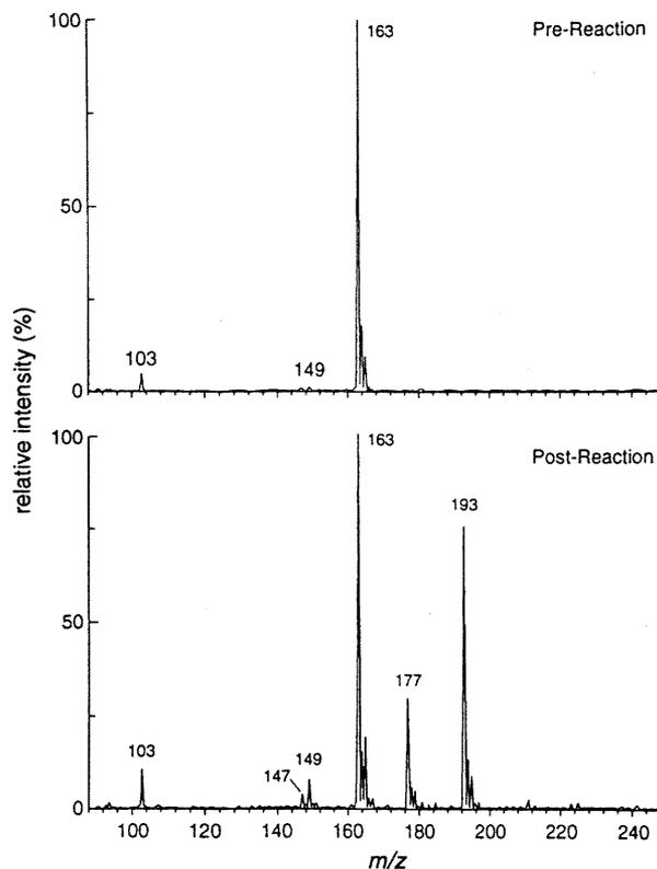
**Fig. 2** API MS spectra before and after irradiation of a  $\text{Cl}_2$ -hexamethyldisiloxane-air mixture for 2.0 min
