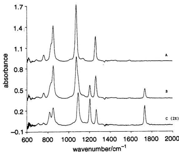
Fig. 4 IR absorption spectrum from the photolysis of a  $\text{Cl}_2$ -hexamethyldisiloxane-air mixture. A, Initial hexamethyldisiloxane,  $7.2 \times 10^{13}$  molecule  $\text{cm}^{-3}$ . B, Reaction mixture after 6 min of irradiation (33% reaction). C, From B after subtraction of unreacted hexamethyldisiloxane. The ordinates of the upper plots are offset for clarity.
