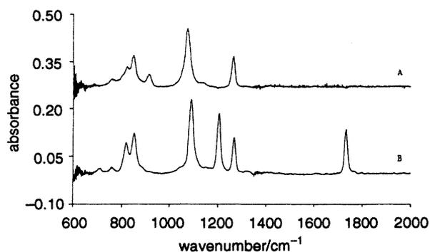
Fig. 5 Comparison of A, the IR spectrum of an authentic sample of  $(\text{CH}_3)_3\text{SiOSi}(\text{CH}_3)_2\text{OH}$  ( $2.4 \times 10^{13}$  molecule  $\text{cm}^{-3}$ ) with B, the IR spectrum of  $(\text{CH}_3)_3\text{SiOSi}(\text{CH}_3)_2\text{OCHO}$  (the same spectrum as in Fig. 4C). The ordinates of the upper plots are offset for clarity.
