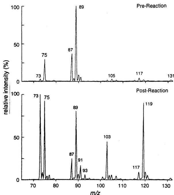
Fig. 7 API MS spectra of a  $\text{Cl}_2$ -trimethylsilylmethanol-air mixture before (top) and after (bottom) irradiation
